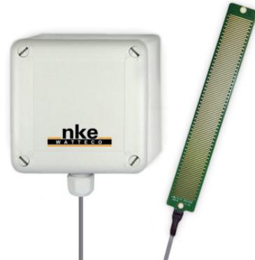
The operating principle is the measurement of voltage variation across the voltage divider bridge formed by the variable resistance probe ( $R = 300 \text{ k}\Omega$  dry,  $R = 2 \text{ k}\Omega$  wet) and the 0-10V analog input of the PRESS'O.
